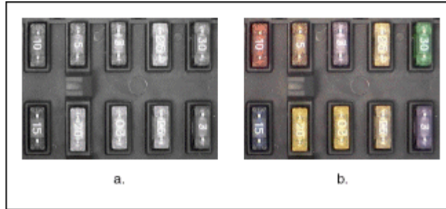
Figure 12. Using Color Pattern Matching to Accurately Identify Objects
